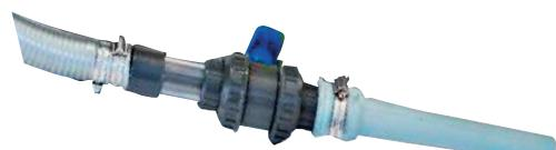
When the tank is empty remove the nozzle from the deck connection and immerse the nozzle a bit into the water. Run the pump again for approx. 10 seconds to flush out the hose. Pull the nozzle out of the water and the vacuum valve shuts off the pump. Return the hose to the pump/Pump-Out station.
