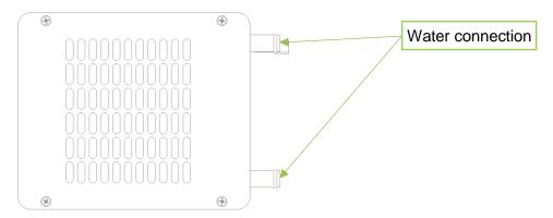
Appropriate set of hoses and hose clamps should be used to connect the product to the system.
