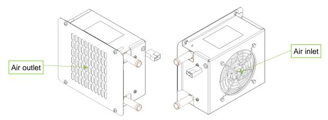
It is recommended to install defroster in a way to ensure that inlet air is filtered. This will ensure longer product life and will prevent defroster from distributing dusty air.
