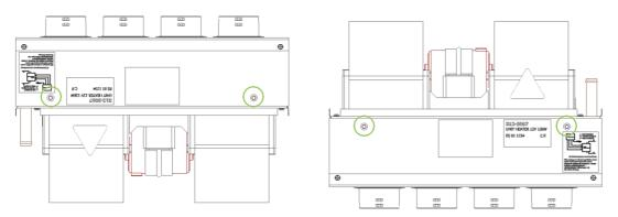
Alternatively,  $\Phi$ 3 mm (0.12") holes on both sides of defroster, combined with adequately sized screws, can be used to mount the unit in place.
