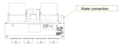
Appropriate set of hoses and hose clamps should be used to connect the product to the system.
