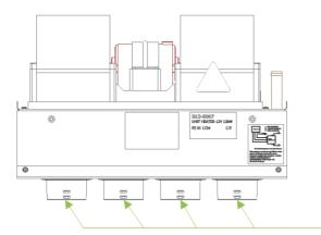
4x connection for  $\Phi 60$  mm (2.4") air hoses, air outlet side
