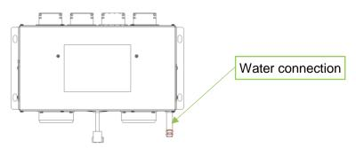
Appropriate set of hoses and hose clamps should be used to connect the product to the system.
