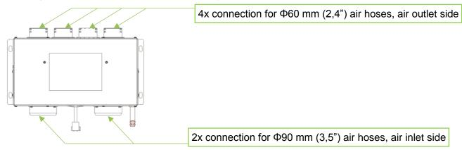
Make sure that air hoses are affixed tightly to adapters by means of adequate clamps to prevent any air leakages and loss of performance.
