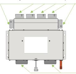
6x connection for Φ63,5 mm (2,5") or Φ60 mm (2,4") air hoses, air outlet side
