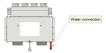
Appropriate set of hoses and hose clamps should be used to connect the product to the system.
